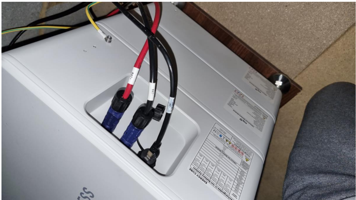
Fig 27. Re connect all cables to the battery module.
