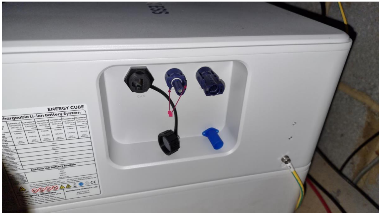
Fig16. Battery terminal clips and CAN cable ports.
