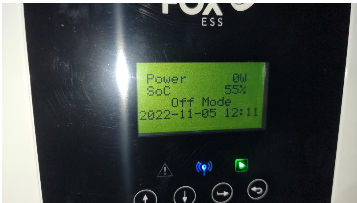
Fig 10. Display showing Power at 0, mode as 'Off Mode'.
