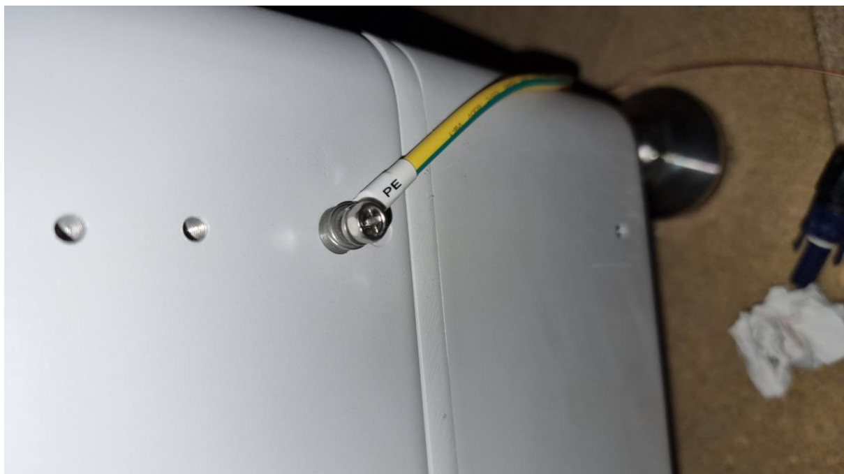
Fig 17. Unscrew the yellow earth cable from Master module.
