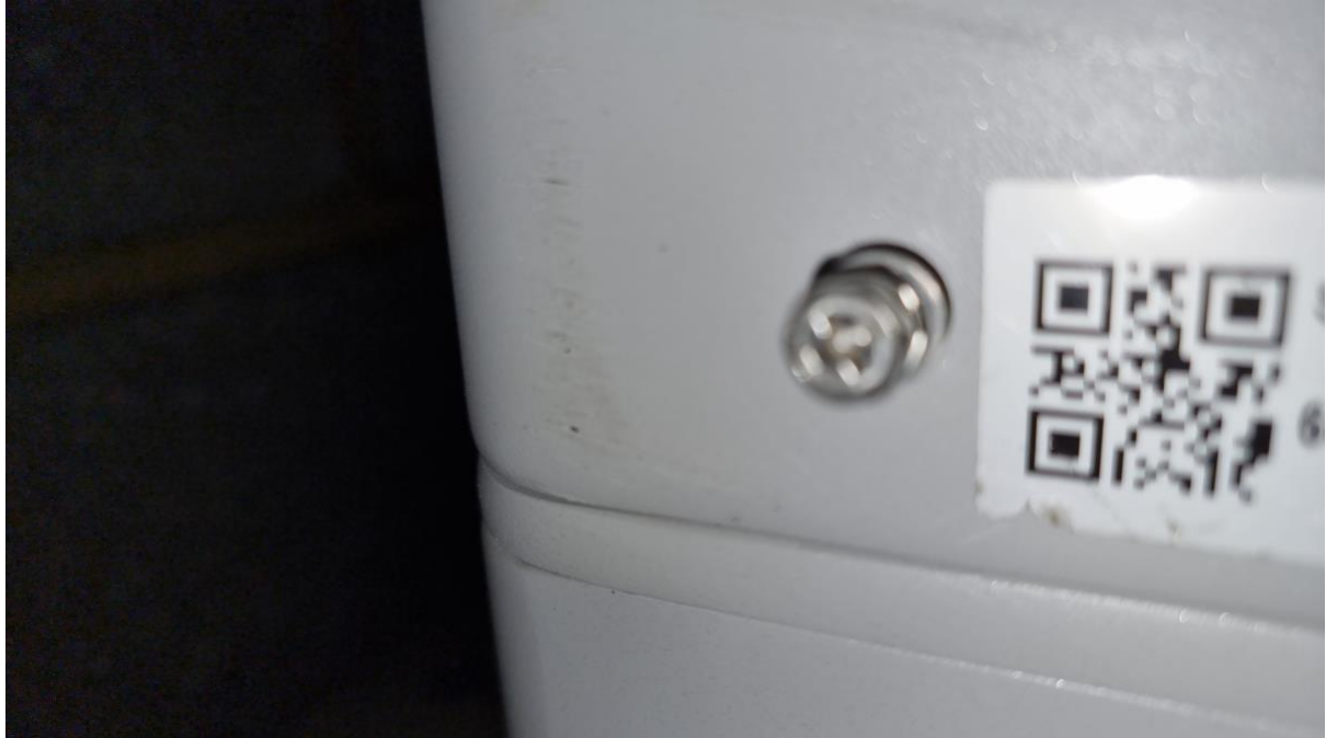
Fig 18. Mounting screw located on the front side bottom left corner.
