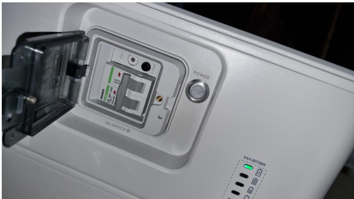
Fig 15. Location of 'Power' button, and unscrew the protective cap to locate DC breaker switch as above. Turn both of these off, you should see no LEDs lighting up.
