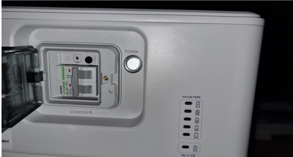
Fig 32. Battery module turned 'On'.
